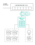
If looking to utilize excess capacity on existing panels which have other loads, we'll install electrical sensors to take advantage of the available capacity at every moment in time. This enables even more chargers to be installed to avoid additional infrastructure costs.
